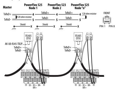
**IMPORTANT** The shield is connected at ONLY ONE end of each cable segment.
