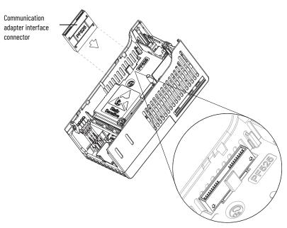
2. Align the connectors on the communication adapter to the communication adapter interface connector, then push the back cover down.
