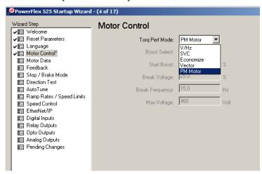
This configuration can also be done by setting parameter Po39 [Torq Perf Mode] to 4 "PM Motor".
