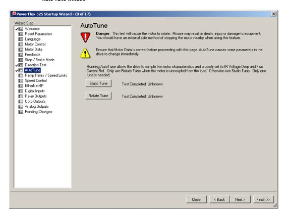
A properly tested motor and drive helps ensure higher starting torque and better performance at low speeds. Conversely, an improperly performed Auto Tune can cause the motor to exhibit instability at low speeds, uneven performances when running through the motor speed range, and can generate unnecessary faults such as overcurrent and overvoltage faults.
