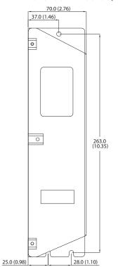
Filter can be mounted onto the back of the drive.
