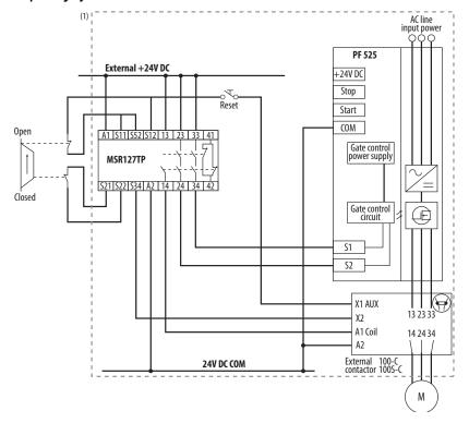
(1) Enclosure Recommended. External wiring failure modes must be considered as described in EN ISO 13849-2. Enclosure or other measure to exclude these failure modes should be used.
