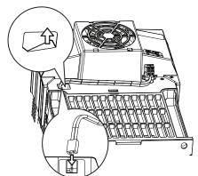
**IMPORTANT** Remove the label to access the built-in 24V supply on drive frames D and E for use with the Control Module Fan Kit.
