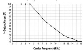
Note: If Vector mode (open loop) is selected and 16 kHz is selected, the drive forcibly reduces the carrier frequency to 8 kHz.
