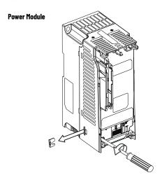
**IMPORTANT** Tighten screw after jumper removal.
