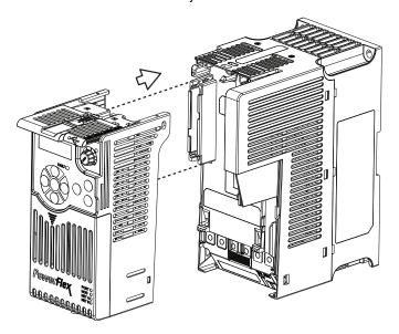
2. Push the top cover of the Control Module towards the Power Module to lock it.
