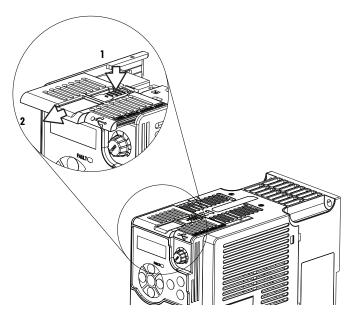
3. Hold the sides and top of the Control Module firmly, then pull out to separate it from the Power Module.
