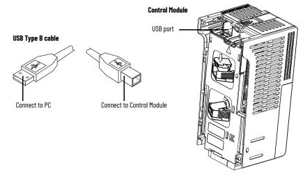
When connected, the drive appears on the PC and contains two files:
