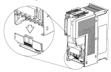
Reattach the terminal guard when wiring is complete.
