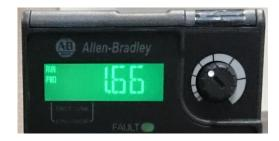
In Connected Components Workbench software, parameter bo10 [Process Display] and bo11 [Process Fract] are shown separately.
