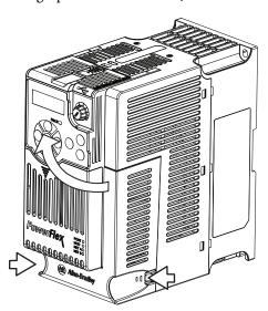
2. Press and hold down the locking tab on the terminal guard.
