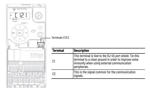
Connect terminal CS1 or CS2 to a clean ground when using a network with a ring topology.
