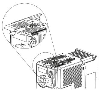
3. Insert the catch at the top of the frame cover into the Power Module, then swing the frame cover to snap the side catches onto the Power Module (Frames B...E only).
