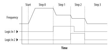
The step time value and the basic logic may be used together to satisfy machine conditions. For instance, the step may need to run for a minimum time period and then use the basic logic to trigger a transition to the next step.
